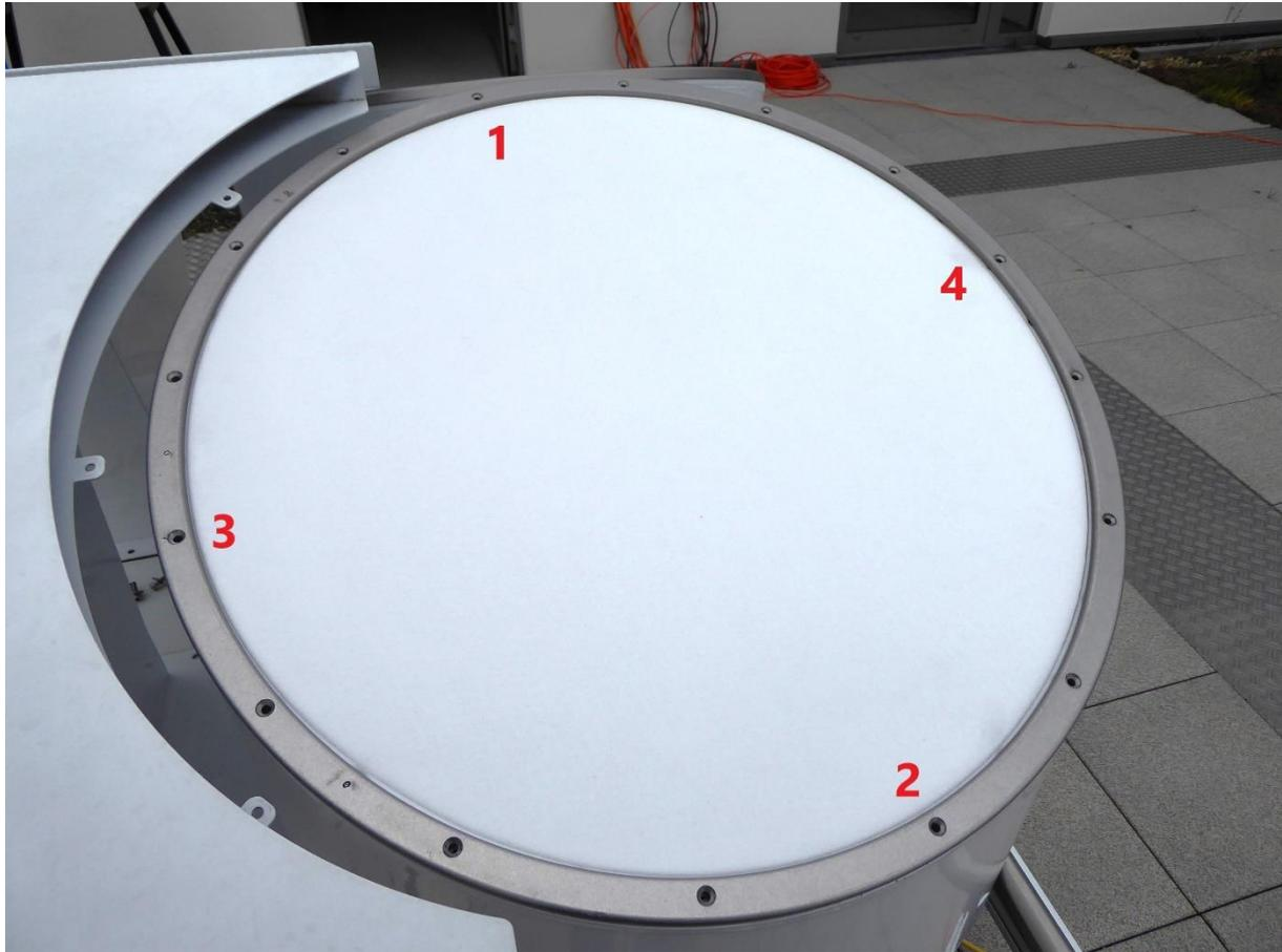
When all the screws are tightened, cut off the material outside the ring with a sharp knife.
