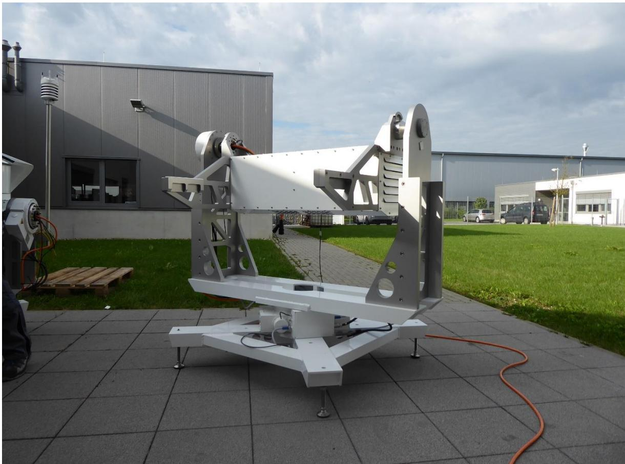
***Unpacked scanner of the dual frequency 35 / 94 GHz cloud radars.***
