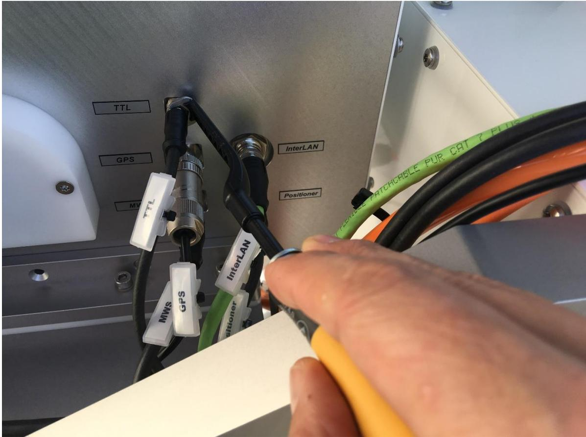
***W-band radar sidewall with connecting cables.***
