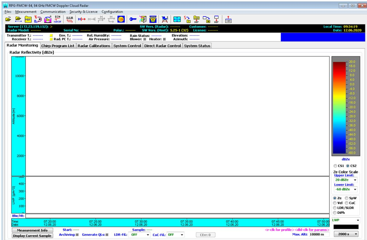
The screen is showing the **Radar Monitoring** tab. On top of the tab, environmental parameters (surface sensor data), position and blower status are displayed. The black panel summarizes the radar ID information, as model number, polarisation, customer code, software version and license status.
