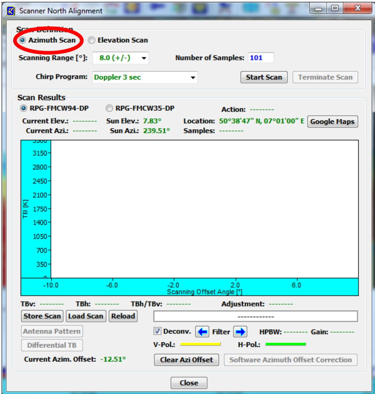
It should be clear that a solar scan is only possible during day time and without any obstacles in the direction of the sun. If the sun is at low elevation, only azimuth scans should be used (as indicated above) because a scan in elevation would drastically change the airmass and therefore the atmospheric damping over the scan.
