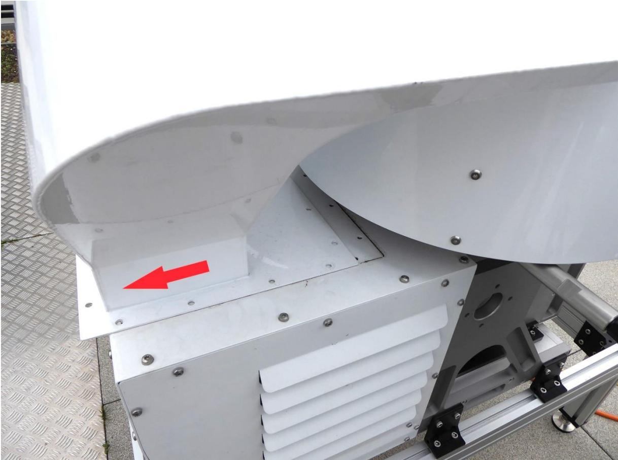
Unscrew all 16 screws holding the radome.
