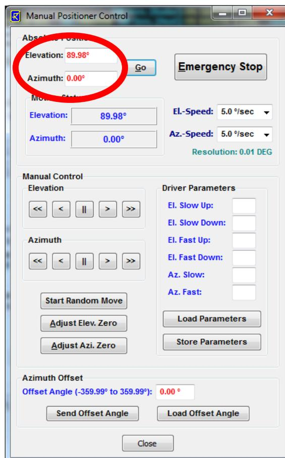
Enter the numbers in red and click on **Go**. The scanner should move to zero azimuth direction. Then switch to the **System Status** tag:
