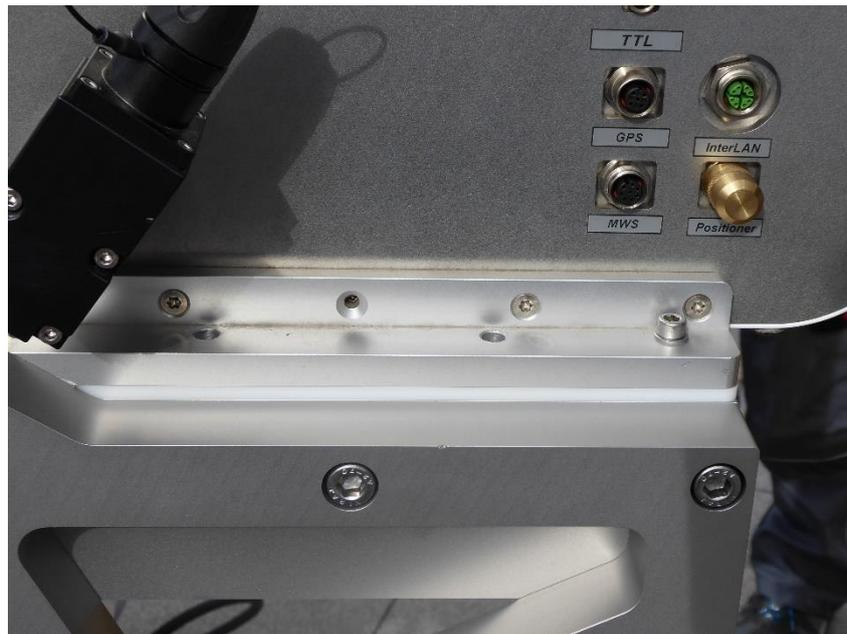
Fasten the K-band radar the same way as done with the W-band radar. Use a total of M6 x 35 screws and tighten them properly. Then connect the InterLAN, power and data cables. Make sure that all non-connected sockets on the radar's side wall are protected with plastic caps:
