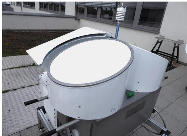
Repeat the steps for the other antenna and reinstall the air guides.
