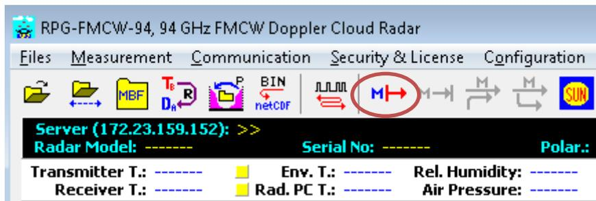
When an MDF or MBF is loaded (**Load MDF/MBF File**), its contents and repetition factor are displayed. In addition some pre-checks are performed, e.g. radar configuration, MDF version number, availability of chirp program number, etc. A variety of other checks ensure that no erroneous command data is sent.
