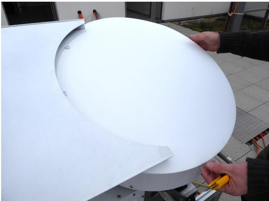
Put the metal ring on the radome sheet.
