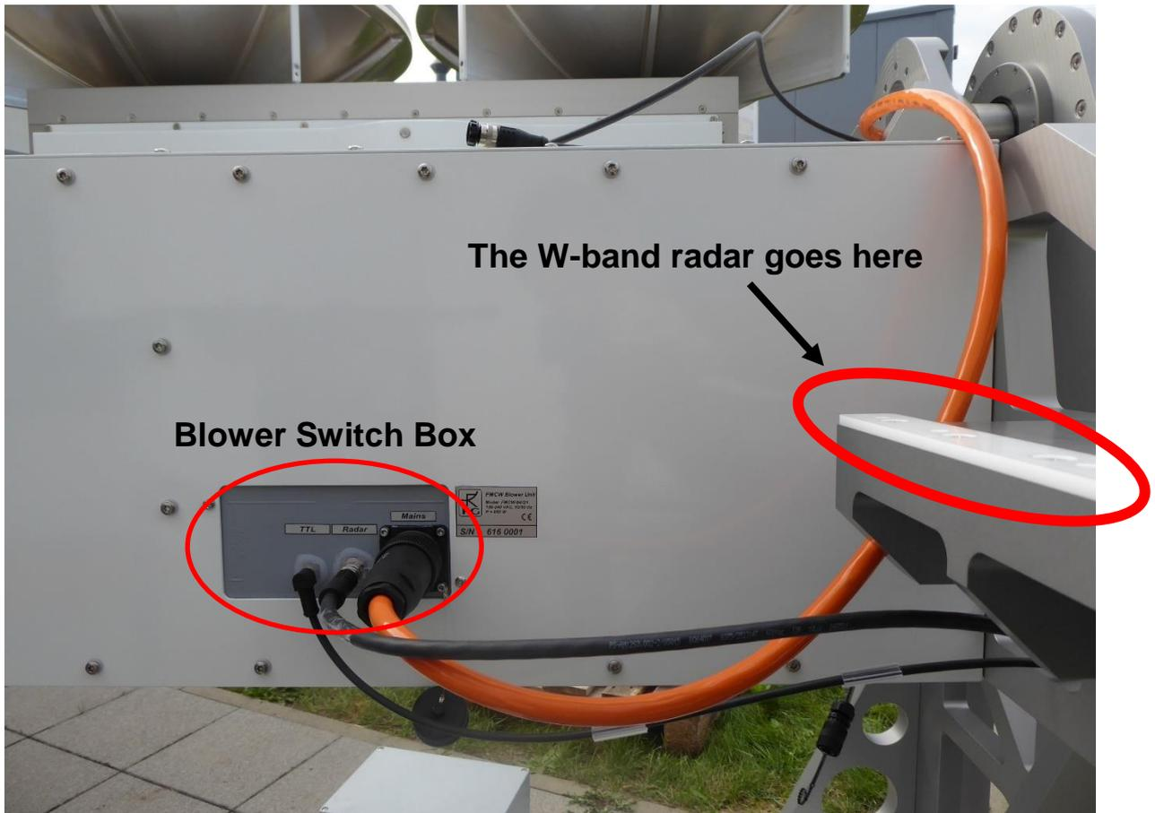
***Make sure that no cables are lying on the radar mounting surfaces while lowering the radar onto the white plastic sliding bars.***
