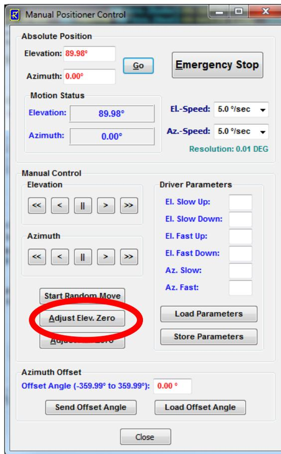
The scanner's elevation zero is now set to the old  $-0.1^\circ$  position. When you return to  $90^\circ$  elevation, the inclination sensor's elevation reading should be close to zero now.
