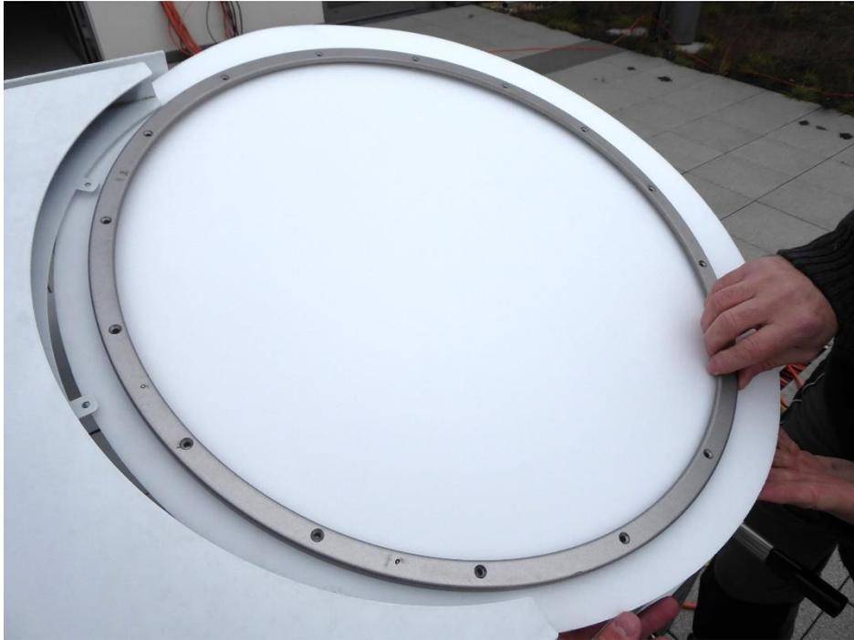
Punch the radome material with one screw through one of the ring holes and screw it down lightly.
