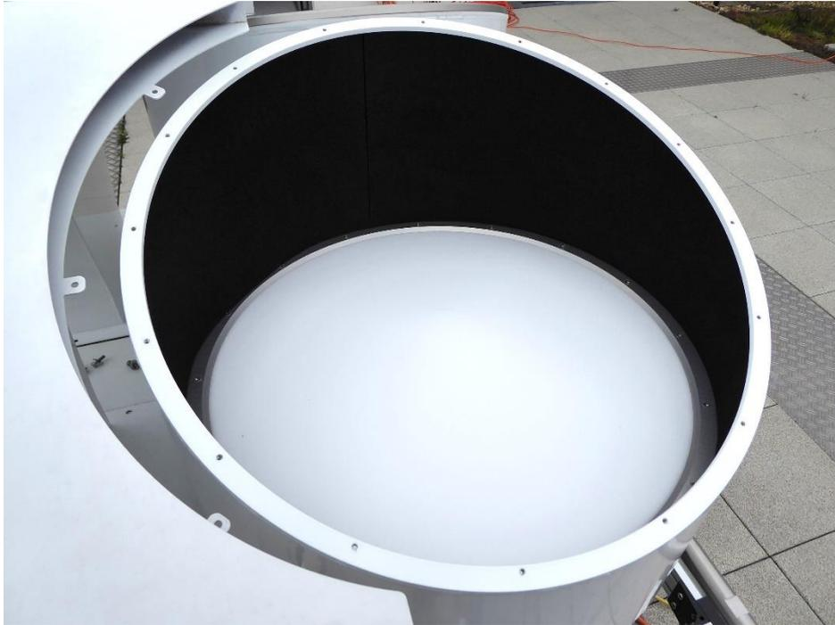
Put a new radome sheet on the cylinder. Make sure the coated (rough) side is facing upwards.
