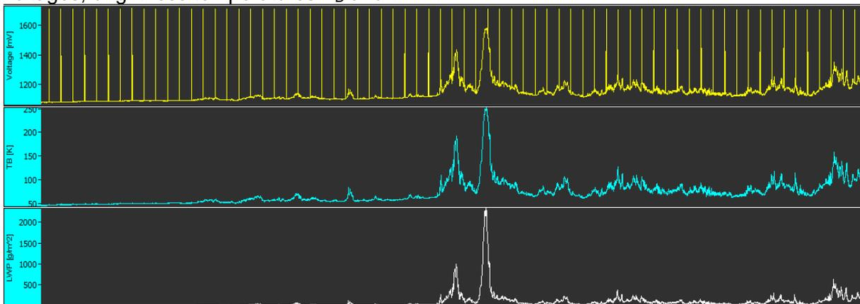
Additionally, information about the IF power level at the ADC board input (end of IF chain) as well as the transmitter power level are presented. The later one demonstrates the automatic power levelling during periods of strong reflections intended for preventing receiver saturation:
