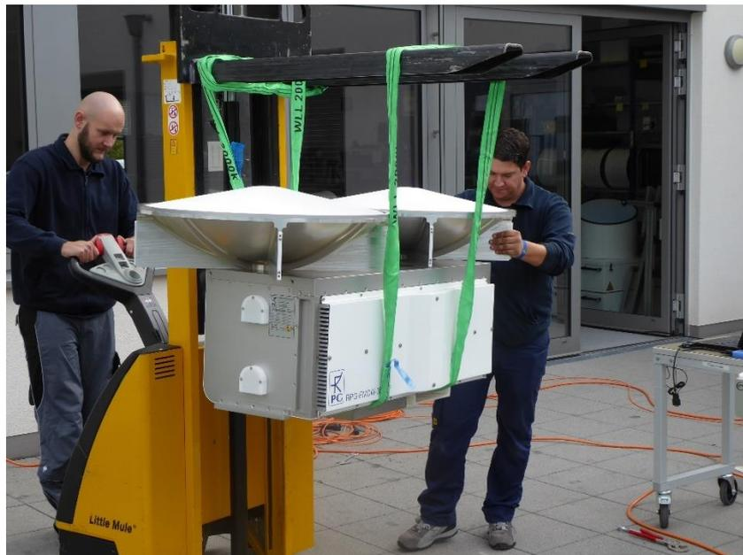
The connectors must point to the **LEFT** when lowering the radar onto the scanner, thus the opposite as for the W-band radar.
