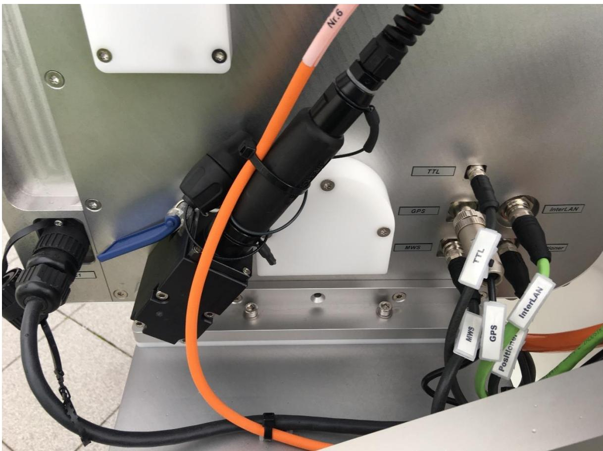
***Please do not apply strong force when screwing the connectors onto the sockets and also do not use pliers. This may lead to damages of the connector pins.***
