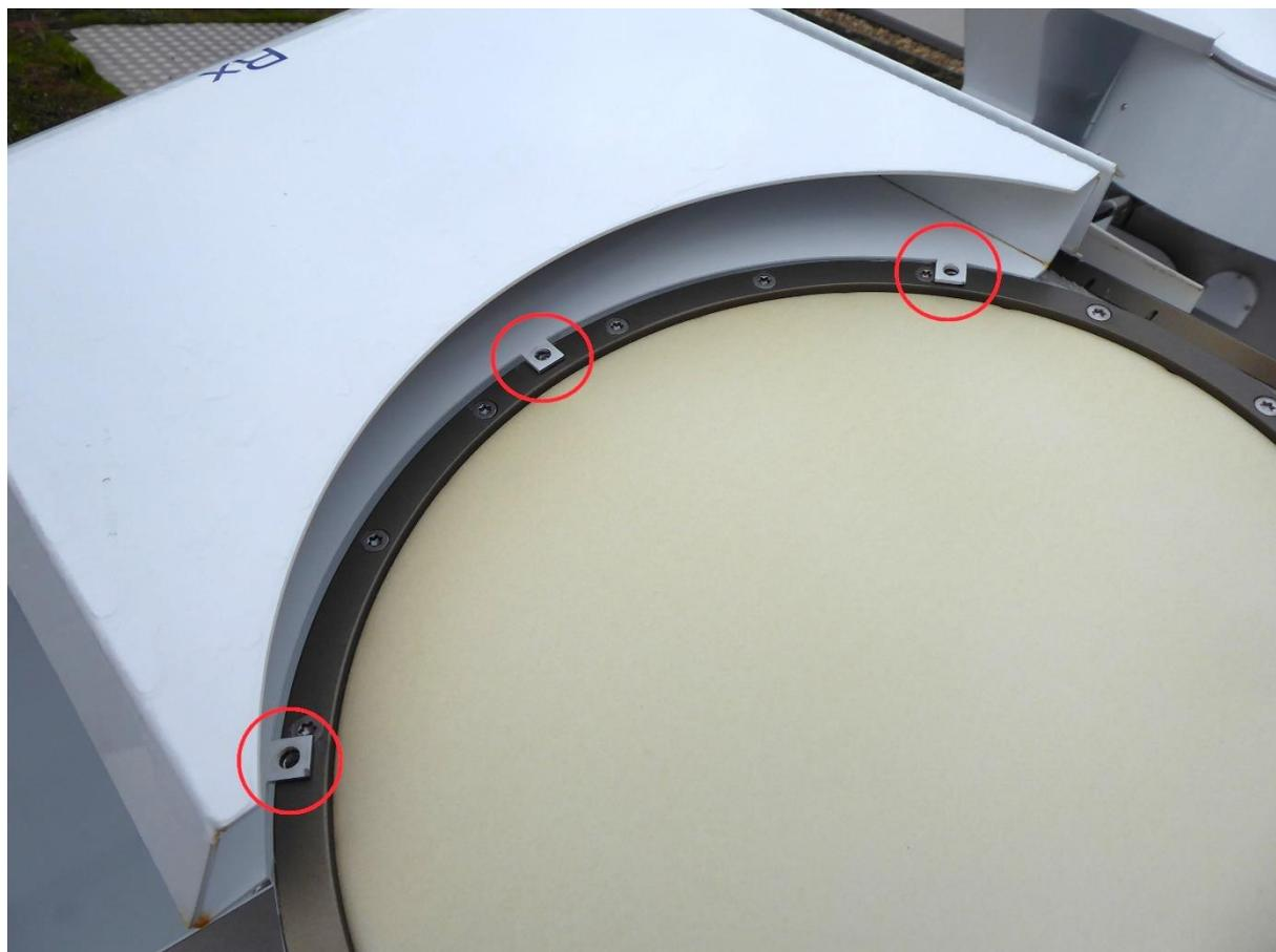
Remove all the screws holding both air-guides.
