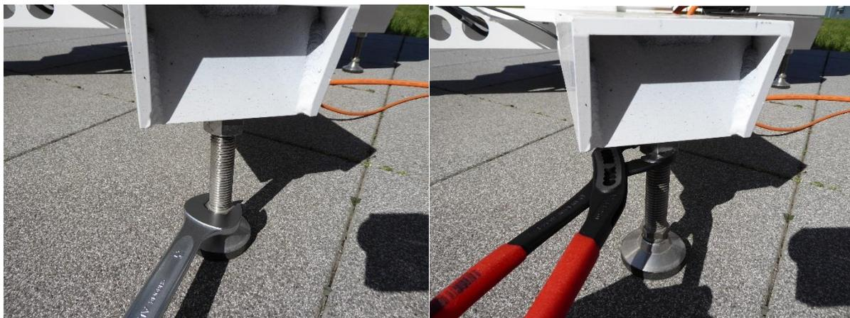
**Use the elevation axis tilt reading for the horizontal alignment in both directions.**
