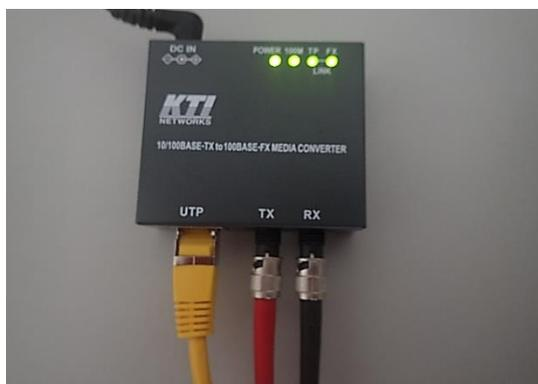
***2-line fiber optics to LAN-TCP/IP converter.***
