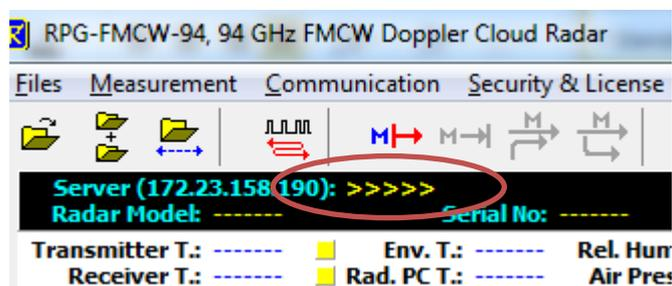
The Host assumes a radar (Server) with a certain IP connected to the network or directly connected (peer-to-peer connection). This IP is defined on the **System Control** tab in the **TCP / IP** box:
