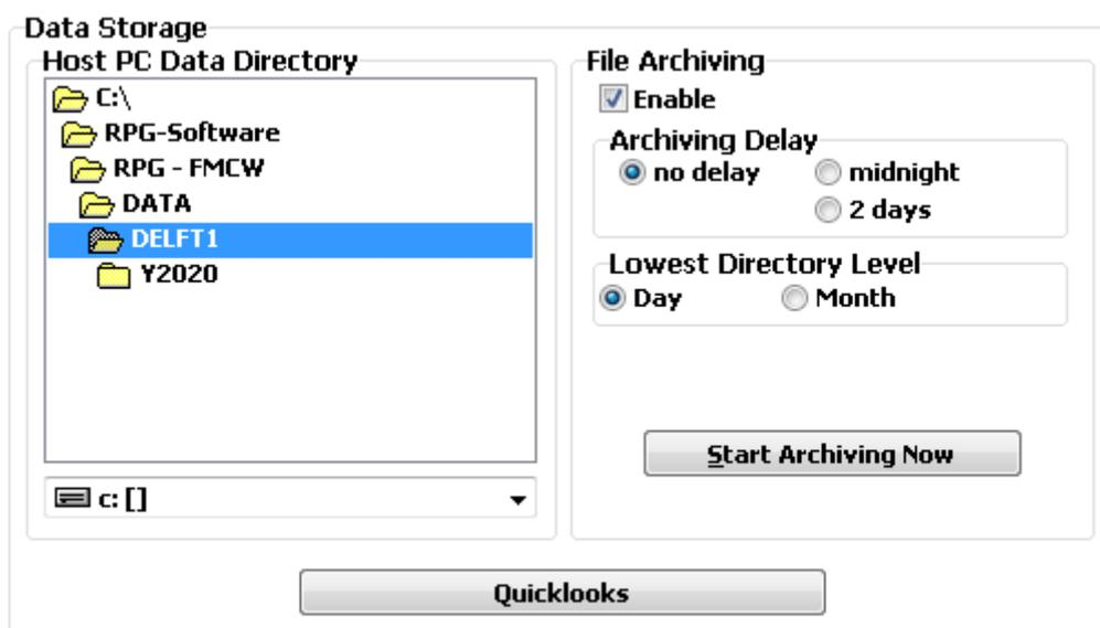
During measurements the recorded radar data is automatically stored in binary format to the directory selected in the **Host PC Data Directory** box.
