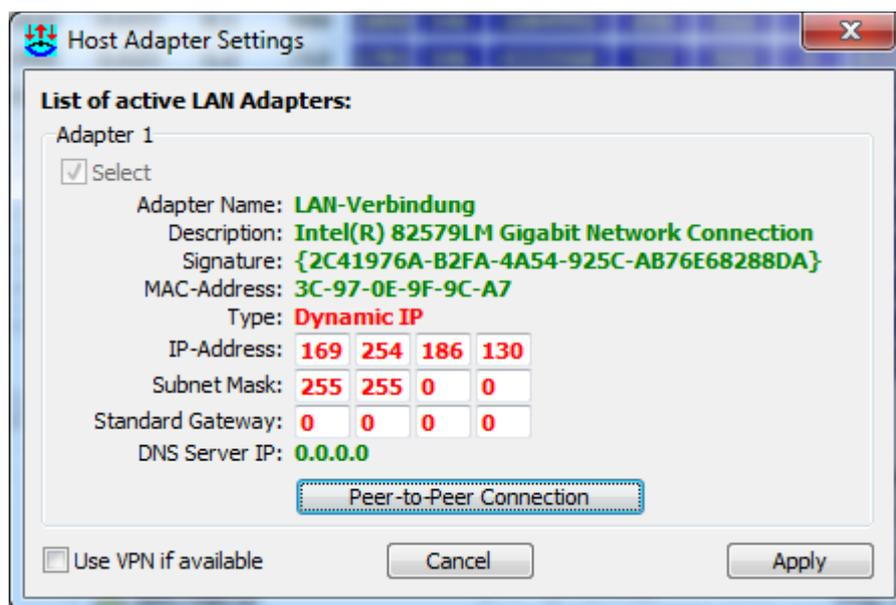
If the IP address you enter here is available within the network the host is connected to, the **Apply** command will automatically change the host IP accordingly. An alternative, of course, is the standard procedure using the Windows IP setting menu.
